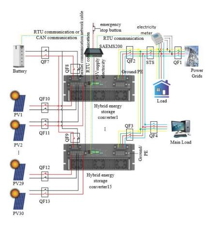
Figure 25 Schematic diagram of parallel connection of single battery packs and multiple machines
