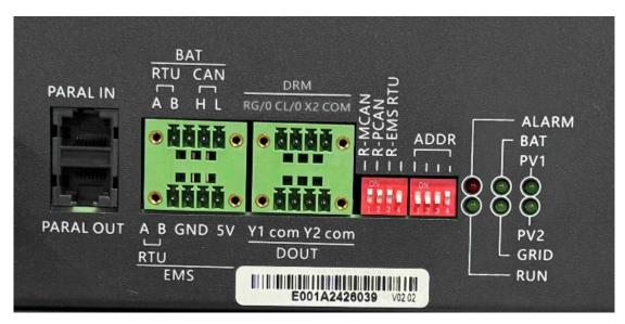
Figure 16 Signal terminal interface definition
