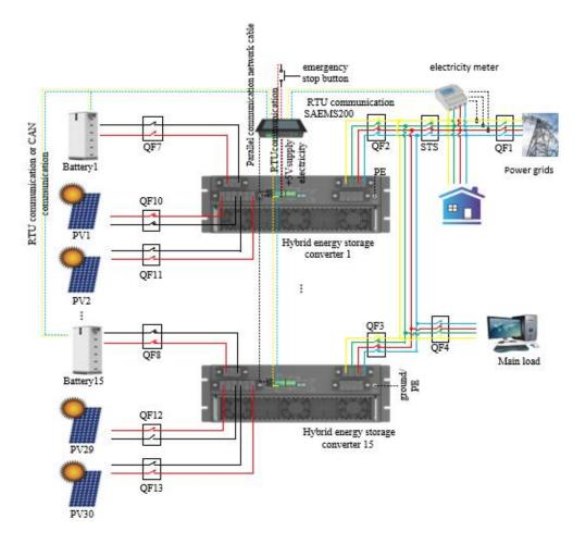
Figure 22 Schematic diagram of parallel connection of multiple machines with one cluster and one management.
