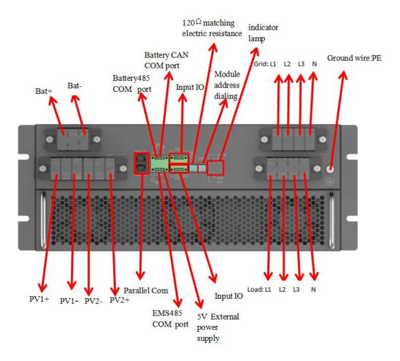
Figure 15 Port Definition Schematic
