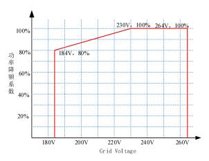
Figure 4 AC charging and discharging power versus grid voltage
