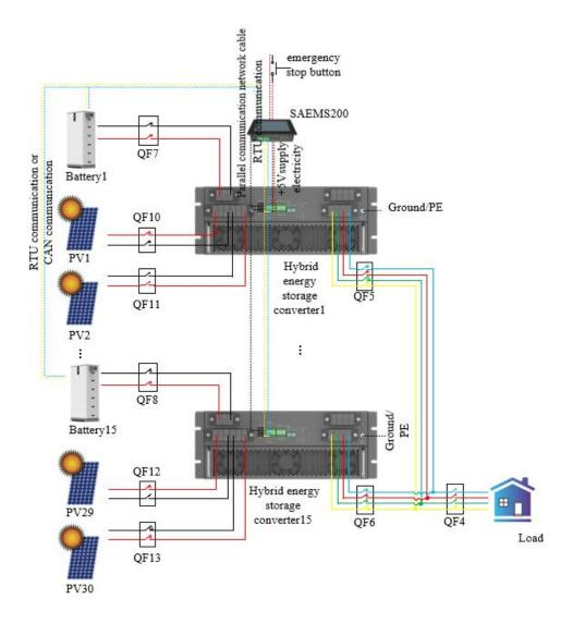
Figure 20 Wiring diagram for parallel connection of multiple machines with one cluster and one manager
