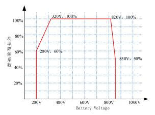
Figure 2 Battery voltage versus discharge power
