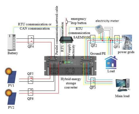
Figure 19 Schematic diagram of one cluster one management wiring
