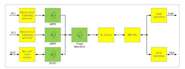
Figure 11 Schematic diagram of power circuit
