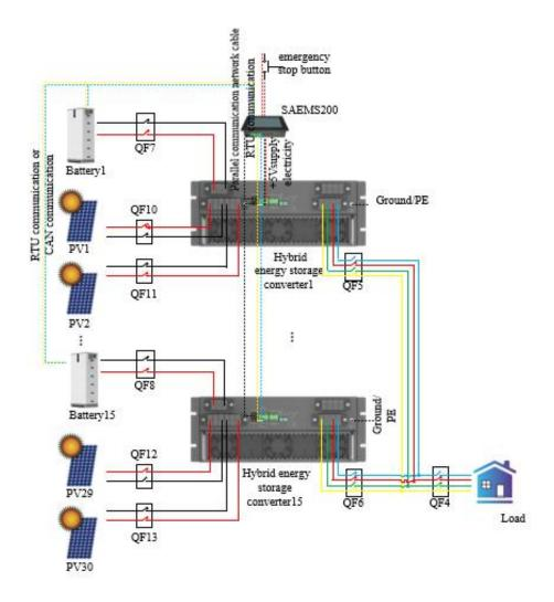
Figure 23 Schematic diagram of parallel connection of single battery packs and multiple machines
