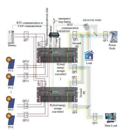
Figure 24 Schematic diagram of parallel connection of single battery packs and multiple machines
