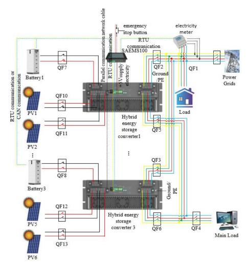
Figure 21 Schematic diagram of parallel wiring of multiple machines with one cluster and one management
