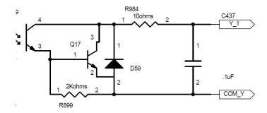
Figure 17 Internal principle of the output trunk node
