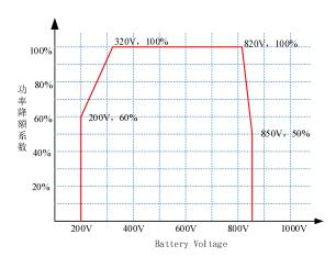
Figure 3 Battery voltage versus AC charging power
