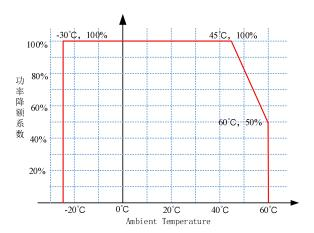
Figure 5 AC charge/discharge power versus ambient temperature
